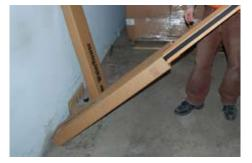
STEP 5 – The rails will need to be opened apart slightly when inserting the other half of the rail box.
