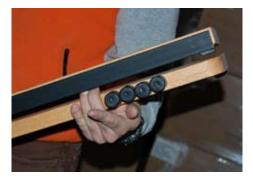
STEP 6 – Position the other half of the rail box so the top edges of the box fit together. Slide the other half of the box down so that the two halves fit together.
